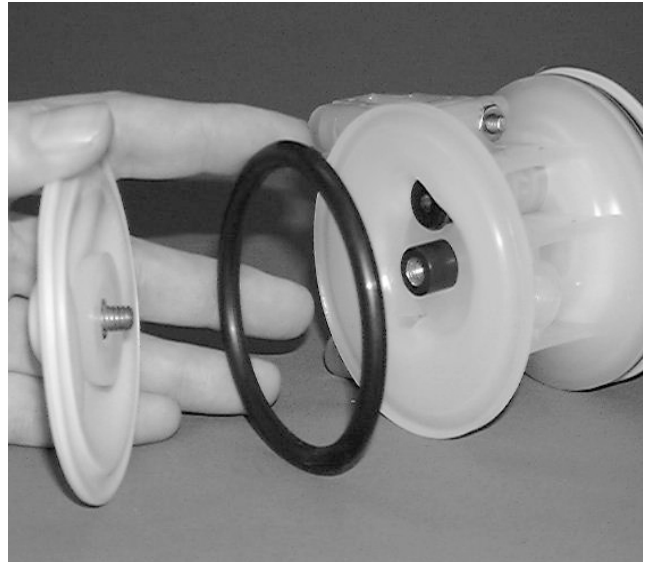
Teflon® diaphragm configuration Figure 2
