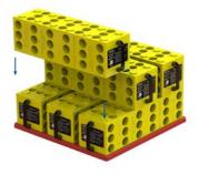
Simply repeat adding layers in alternating directions until the desired height is reached. Up to a maximum of 150cm (60"). Before building the top layer see the next step.
