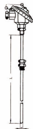
固定卡套螺纹，可动卡套螺纹 Fixed ferrule thread, movable ferrule thread
