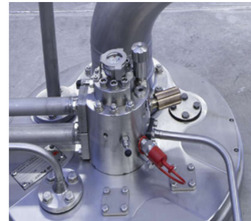
The hydraulic high pressure pipe is located inside the low pressure return oil pipe. The entire hydraulic section is separated from the cargo by a cofferdam ventilated to atmosphere.
