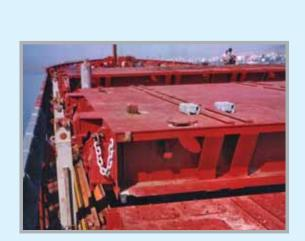
• Hatch covers are manufactured and painted in our facilities and transported to the ship for fitting under the supervision of our engineers. They are produced to be exposed to the severe weather and marine conditions.
