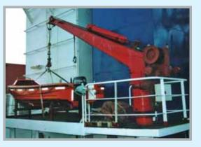
• GÜRDESAN designs and manufactures such cranes that can handle both Rescue Boats-Life rafts and Provisions. Vessels must carry proper cranes for rescue boats and life rafts according to IMO regulations. Characteristics of these cranes are described in Chapter 3 of the international convention for the SOLAS/1974.
