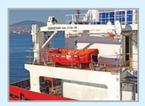
• On all types of vessels or on certain types of specialised vessel, increasing use is being made of deck cranes to perform various lifting tasks. GüRDESAN is achieving considerable success in supplying such cranes to vessels that can conduct both life saving appliance and provision/hose handling work.
