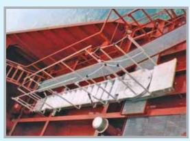
• GÜRDESAN's ladder variety covers Bulwark Ladders, Accommodation Ladders (Shipbuilding – Accommodation Ladders ISO 5488), Gangways (Shipbuilding – Aluminium Shore Gangways for Seagoing Vessels ISO 7061). The characteristics such as lifting capacity, initial sag and deflection under load are tested according to these standards.
